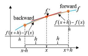
$$egin{aligned} f_x(x,y) &pprox rac{f(x+h,y) - f(x-h,y)}{2h} \ f_y(x,y) &pprox rac{f(x,y+k) - f(x,y-k)}{2k} \ f_{xx}(x,y) &pprox rac{f(x+h,y) - 2f(x,y) + f(x-h,y)}{h^2} \ f_{yy}(x,y) &pprox rac{f(x,y+k) - 2f(x,y) + f(x,y-k)}{k^2} \ f_{xy}(x,y) &pprox rac{f(x+h,y+k) - f(x+h,y-k) - f(x-h,y+k) + f(x-h,y-k)}{4hk} \ \end{aligned}$$
